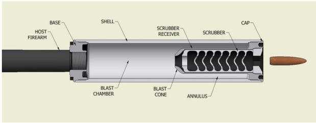
Figure 1: Pantera Components and Features
