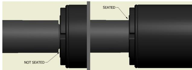
Figure 4: Seating the base to the muzzle thread shoulder.
