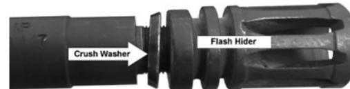
Figure 3: Flash Hider and Crush Washer
